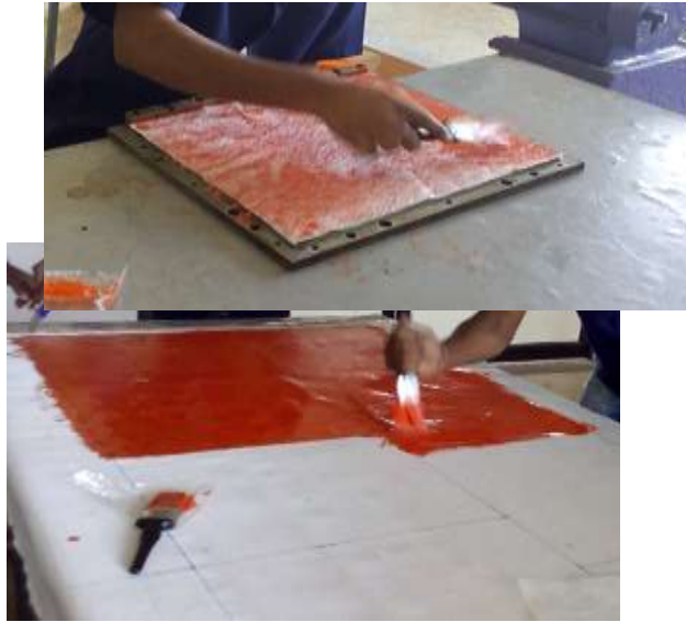
Fig 4.3 applying of plies over mould by sequence
