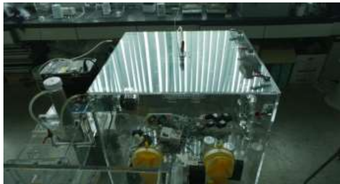
Fig. 7. Methyl methacrylate box made for radon concentration calibration
