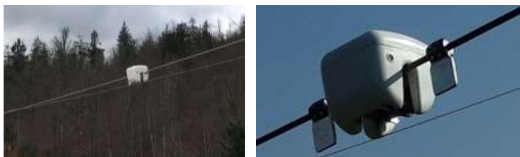
Fig. 4 Installation of OTLM SMART on the conductor & integrated camera [5].
