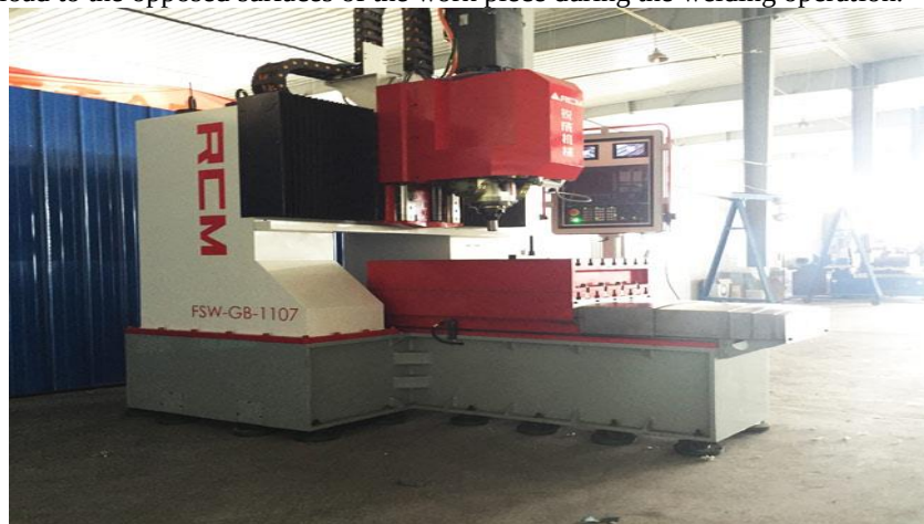
Fig.3. Experimental set up of FSW in BARC
