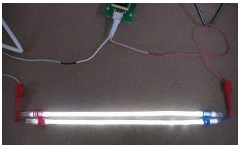
Figure 1 Photopicture of prototype of coil-EEFL lamps in parallel connection. Coil-EEFL lamps are converted from the commercial CCFL lamps.
