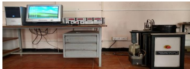
Fig. 2: Pin-on-disc Setup and Wear Monitor
