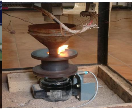
Fig 2. Vertical Centrifugal setup
